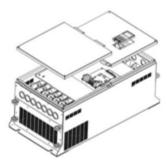
Figure 3-3 Disassembly drawing of lower cover plate of metal plate shell
