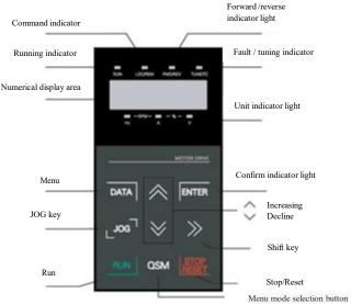
Figure 4-1 Schematic diagram of operation panel
