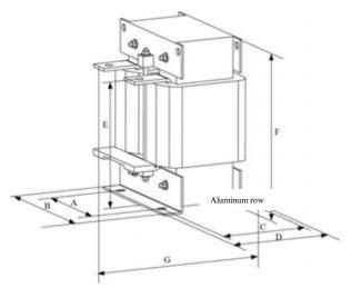
Figure 2-8 Dimensional drawing of external DC reactor
