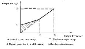
Figure 6-3 Diagram of manual torque boost
