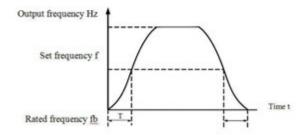
Figure 6-12 S-curve B schematic
