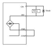
Figure 3-11 Wiring diagram of digital output terminal
