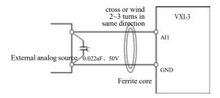
Figure 3-8 Treatment wiring diagram of analog input terminal
