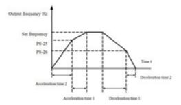
Figure 6-19 acceleration and deceleration time switch schematic
