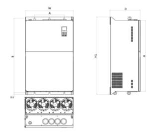
Figure 2-5 Schematic diagram of external dimension and mounting dimension of VXI-3 metal plate structure
