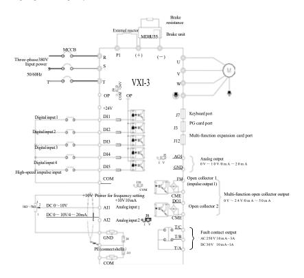
Figure 3-4 Wiring diagram of frequency convertor
