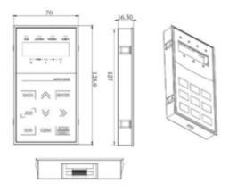
Figure 2-6 External dimension of display panel
