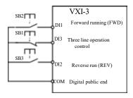
Figure 6-8 Three wire control mode 1
