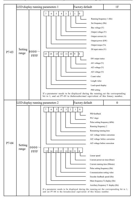
These two parameters are used to set the parameters that can be viewed when the AC drive is in the running state. You can view a maximum of 32 running state parameters that are displayed from the lowest bit of P7-03.
