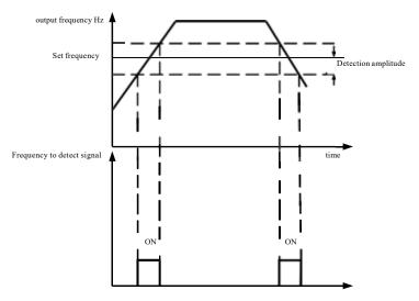
Figure 6-17 Frequency arriving detection amplitude schematic
