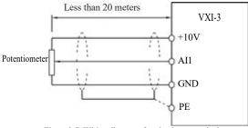
Figure 3-7 Wiring diagram of analog input terminal
