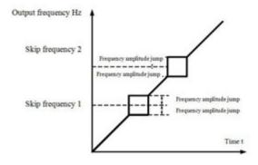
Figure 6-14 Skip frequency schematic
