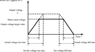
Figure 6-5 Diagram of V/F separation
