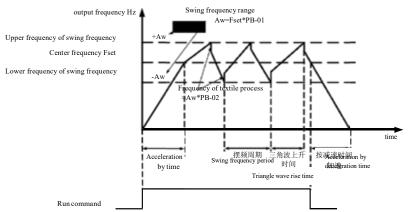
Figure 6-28 Working diagram of frequency swing
