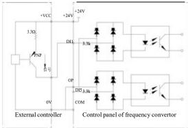
Figure 3-10 Source-type wiring way
