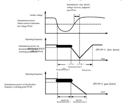
Figure 6-24 Schematic diagram of instantaneous power failure
