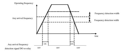
Figure 6-20 arbitrary frequency detection arrival schematic
