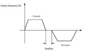
Figure 6-15 Reversible schematic dead time
