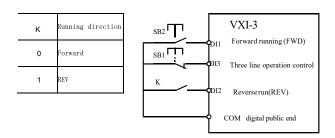
Figure 6-9 Three wire control mode 2
