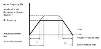
Figure 6-1 Diagram of aceleration and deceleration time
