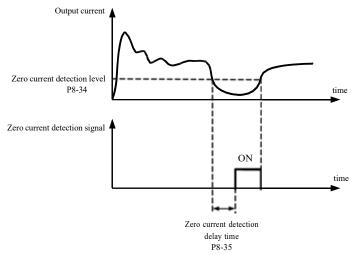
Figure 6-21 Zero current detection schematic
