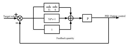
Figure 6-25 Principle block diagram of process PID
