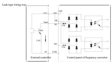
Figure 3-9 Leak-type wiring way
