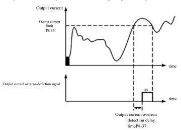
Figure 6-22 Output current limit detection schematic
