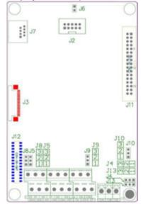
Figure 3-6 Location diagram of jumper and auxiliary terminals
