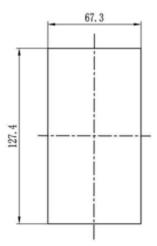
Figure 2-7 Hole size of display panel
