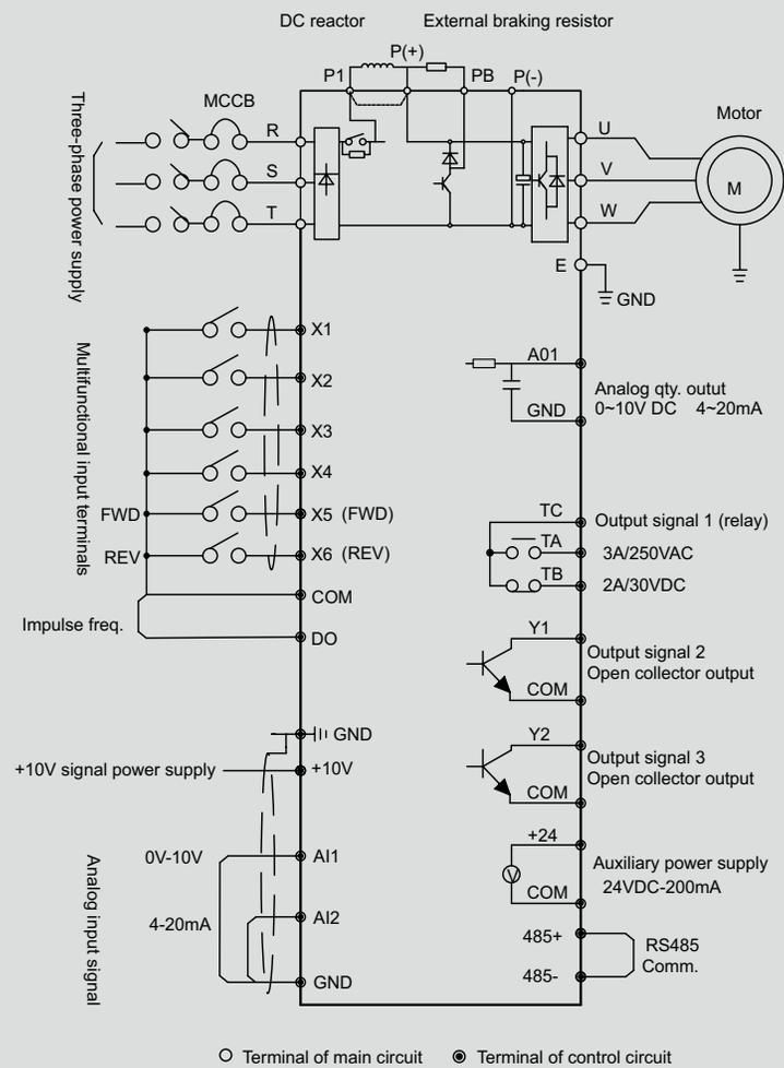
Basic wiring schematic of FC
