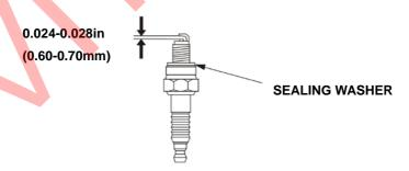
7. Check that the spark plug sealing washer is in good condition,
