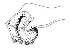
air guide and the air cleaner case with a moist rag, then reinstall
